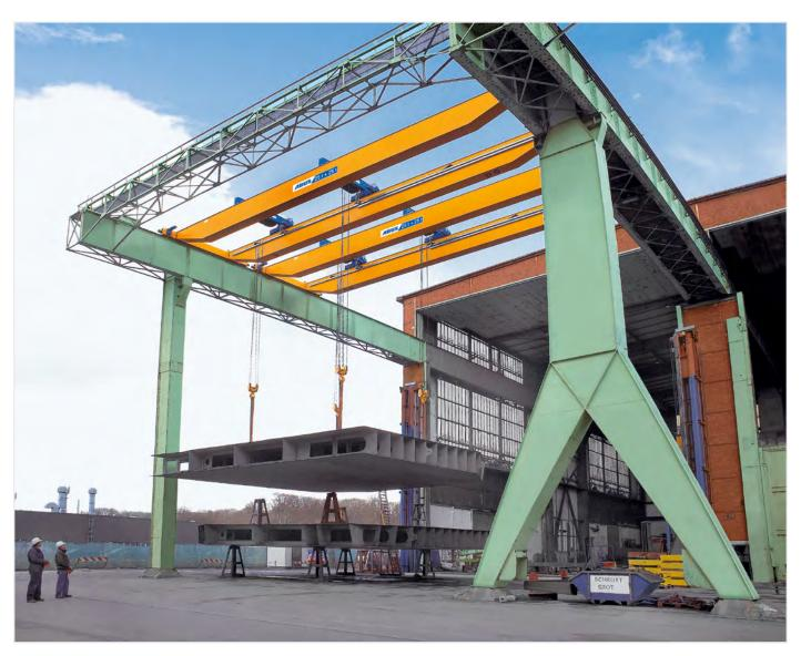
ABUS ABUControl tandem control offers the safest solution for this particular logistical challenge. It makes it possible to move two cranes simultaneously via radio remote control. The operator can choose his optimal location according to the actual operating conditions.
